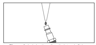
Figure 2. Lubricating directly into air fitting.
